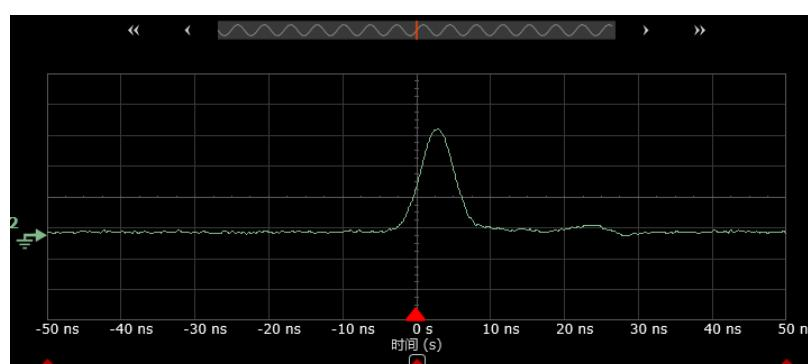
(pulse width : 5ns, rise time : 3ns, fall time : 4ns, repetition frequency : 100KHz)
